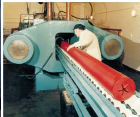
Figure 5-4: A solid propellant extruder and grain.
